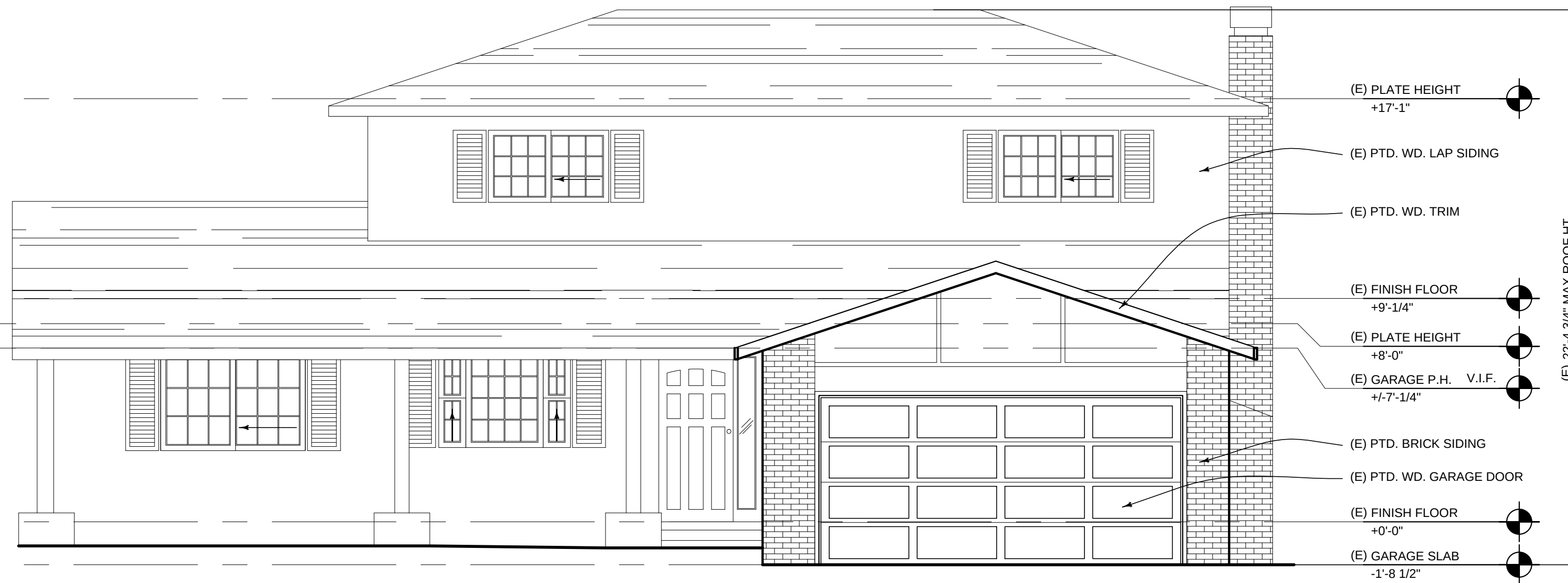
2 EXISTING EAST (FRONT) ELEVATION A3.1 1/4"=1'-0"
