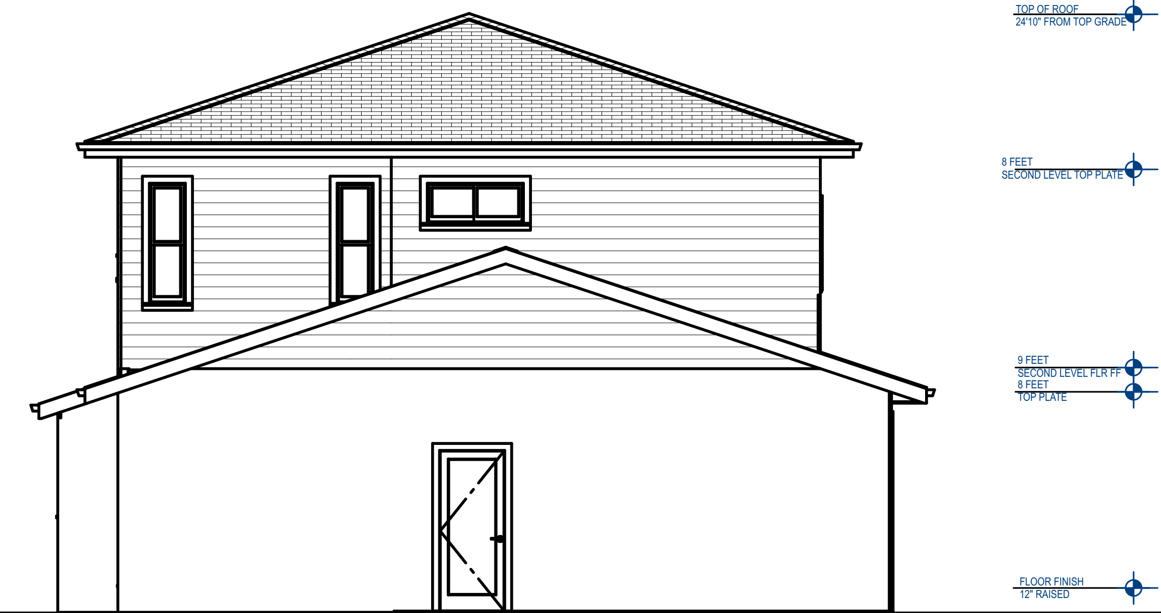
PROPOSED LEFT ELEVATIONS SC : 1/4" = 1'-0"
