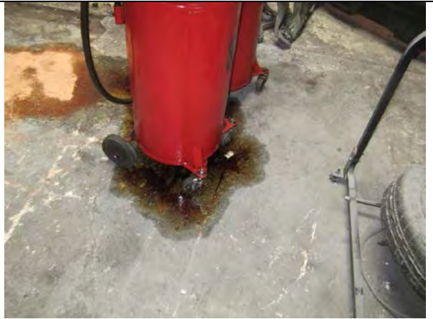
Leaking drum in back storage room of Swedish Auto Service
