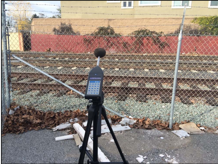
Railroad Noise Measurement Site 1 (note barrier on opposite side of tracks)
