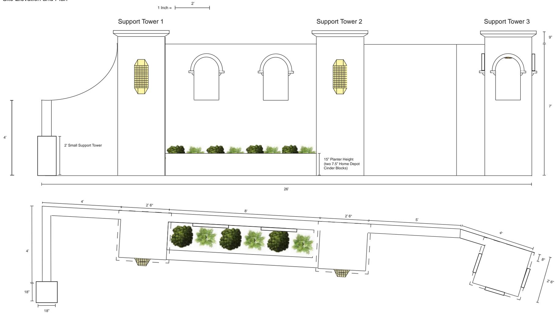
**Materials:** Concrete Base, Cinderblock Walls (Rebar), Some Galvanized Steel Tube Framing, Stucco Walls
